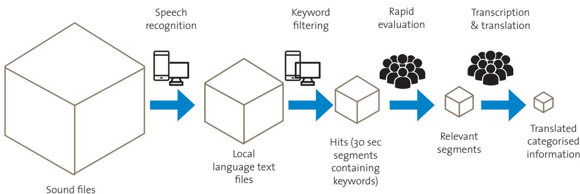
Overall radio mining process for converting a large quantity of unstructured audio data into a small quantity of relevant, structured information.
